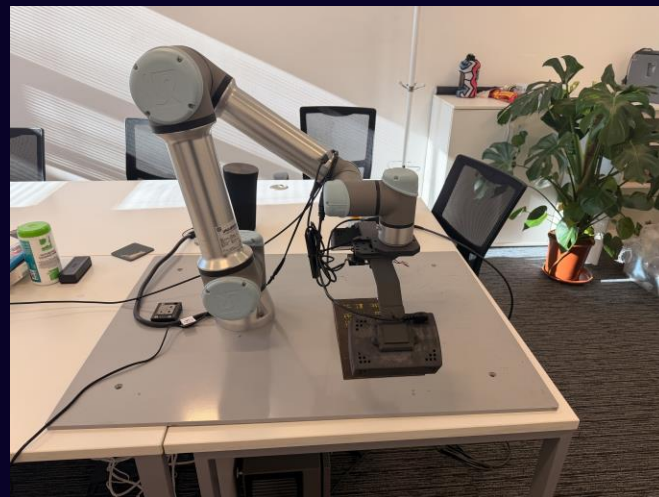
Bullfrog Iris: excitation head, IR camera, and computer integrated onto a Universal Robots cobot arm.
